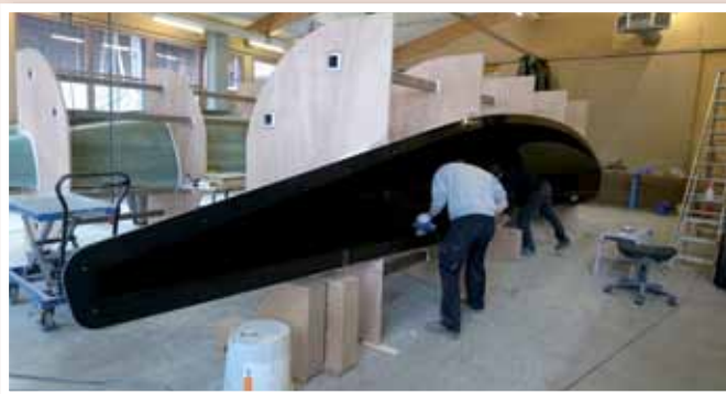
The new plugs are prepared and finished before the two moulds are taken. Finally it is cleaned and polished ready for the first build.
