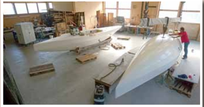
The build process for SUI 229 Momo - The two sides are vacuum infused before being joined together. Below: Checking the weight of bare hull.
