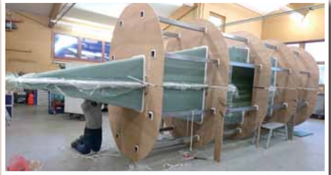
The build process for SUI 229 Momo - The two sides are vacuum infused before being joined together. Below: Checking the weight of bare hull.
