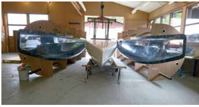
The build process for SUI 229 Momo - The two sides are vacuum infused before being joined together. Below: Checking the weight of bare hull.
