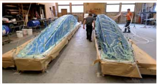
The new plugs are prepared and finished before the two moulds are taken. Finally it is cleaned and polished ready for the first build.
