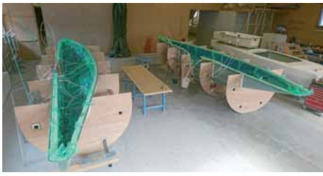
The build process for SUI 229 Momo - The two sides are vacuum infused before being joined together. Below: Checking the weight of bare hull.
