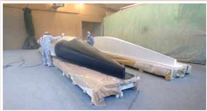
The new plugs are prepared and finished before the two moulds are taken. Finally it is cleaned and polished ready for the first build.
