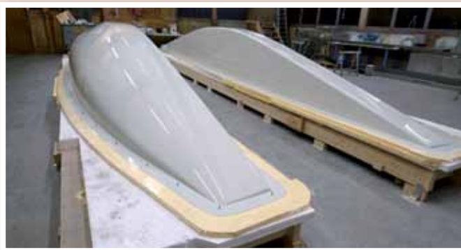
The new plugs are prepared and finished before the two moulds are taken. Finally it is cleaned and polished ready for the first build.
