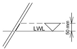
The height of the triangle in the vertical plane shall be not more than 50mm
