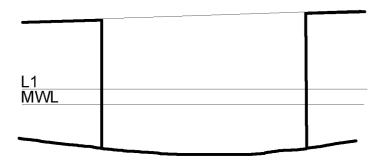
15.5.6 The two watertight bulkheads specified above may be replaced by a watertight cockpit. In this case the cockpit sole shall be above L1 level and the cockpit shall have at least two self bailers. Openings for control lines shall meet the above requirements and any hatches shall maintain the watertight integrity of the cockpit. The weight of each bulkhead, including the weight of the adjacent ring frame if fitted, shall be not less than 6.5kg.
